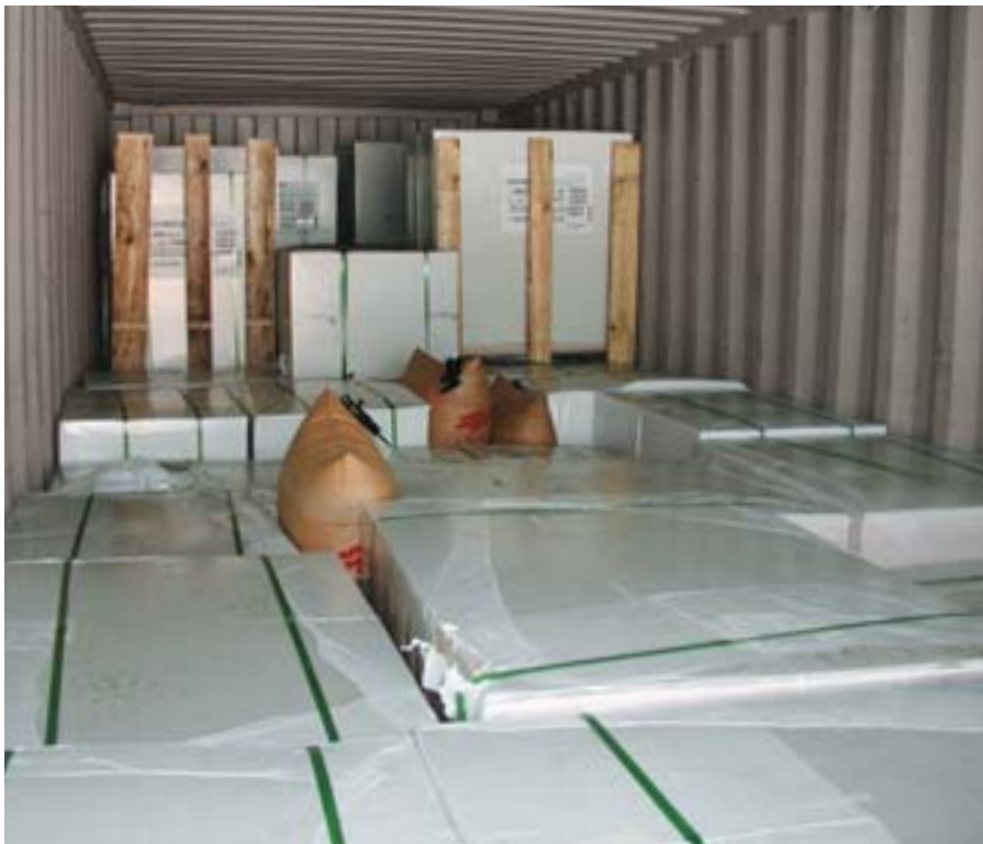
Stowage of non-standard pallets. Spaces are filled with airbags. The pallets in the second layer are each secured with three pieces of dunnage against slipping towards the door
