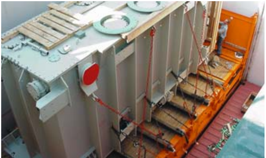
This transformer, weighing approx. 160t, was placed on steel girders and lashed with chains
