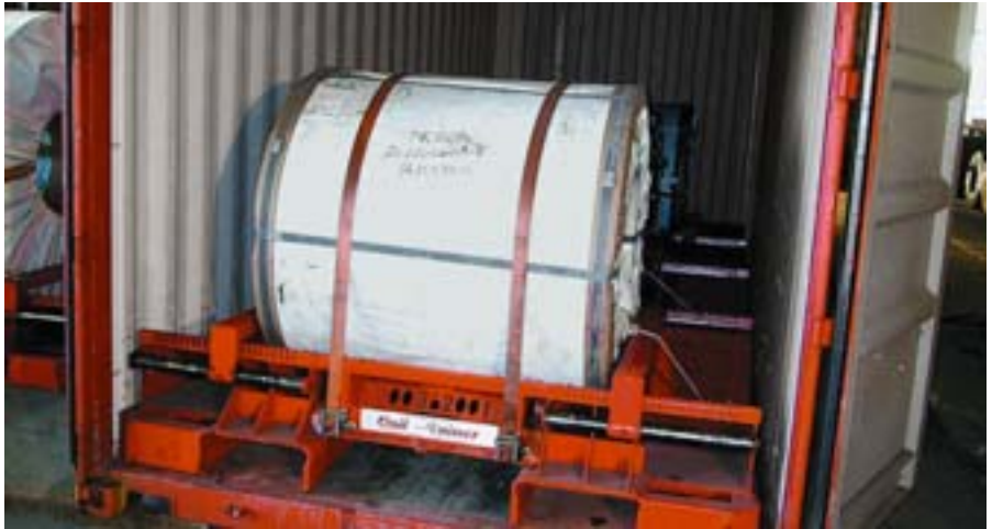
Steel coil secured on a Coil-Trainer cradle
