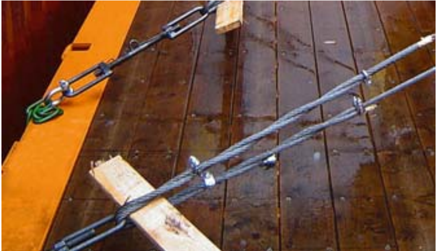
Correct lashing arrangement. The steel wire is twisted to increase the friction
