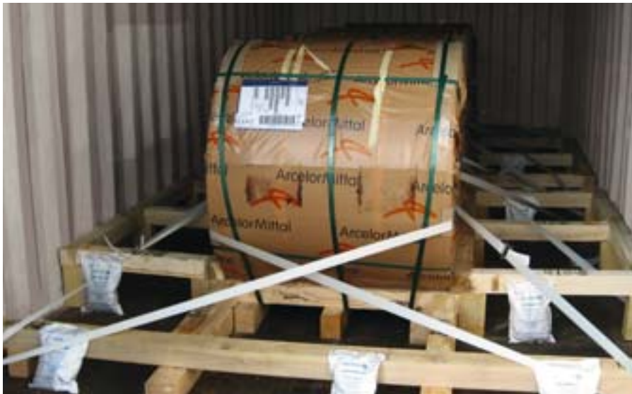
Steel coil loaded with axis across, chocked to the side and lengthwise and lashed with nylon belts
