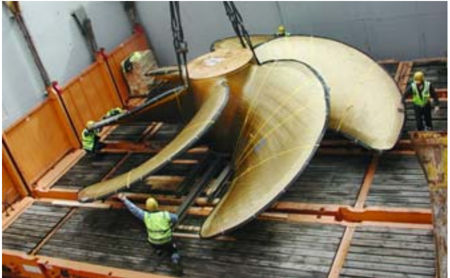
Loading a large ship propeller weighing 80t. The propeller has a very small contact area, so robust steel bedding is used. Additional wooden supports are positioned under every propeller blade and steel wire or straps used for lashing
